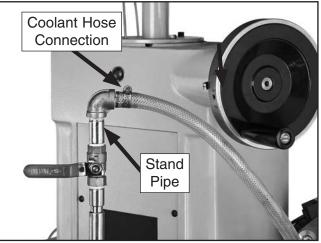
Figure 12. Coolant hose connection to stand pipe.
